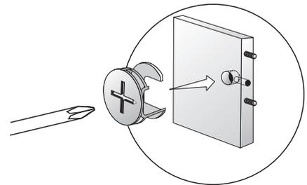
Use a screwdriver to rotate cam into correct alignment.
